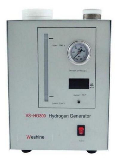
This Hydrogen Generator make the hydrogen for the Gas Chromatography Test, the hydrogen can help to fire the FID1 and FID2.
